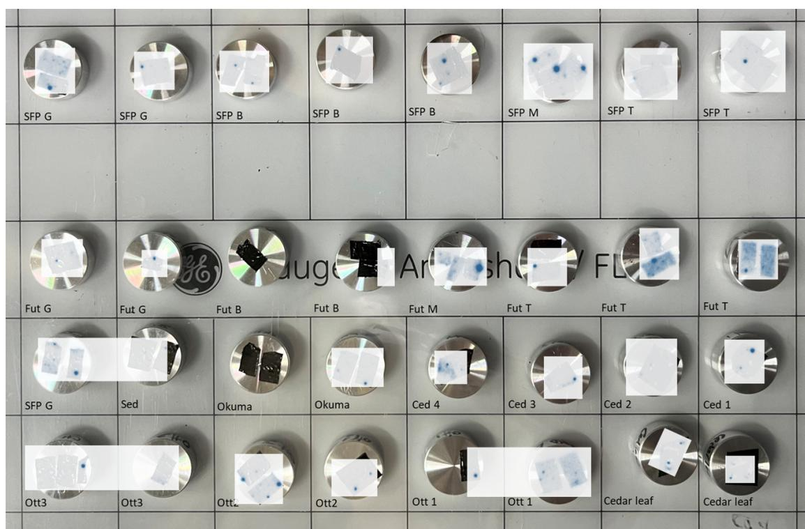
**Figure 3.5:** Hotspots identified with autoradiography imaging isolated onto SEM stubs, labelled with sampling location. The stubs were exposed altogether for a week, showing the relative intensity of the hotspots.
