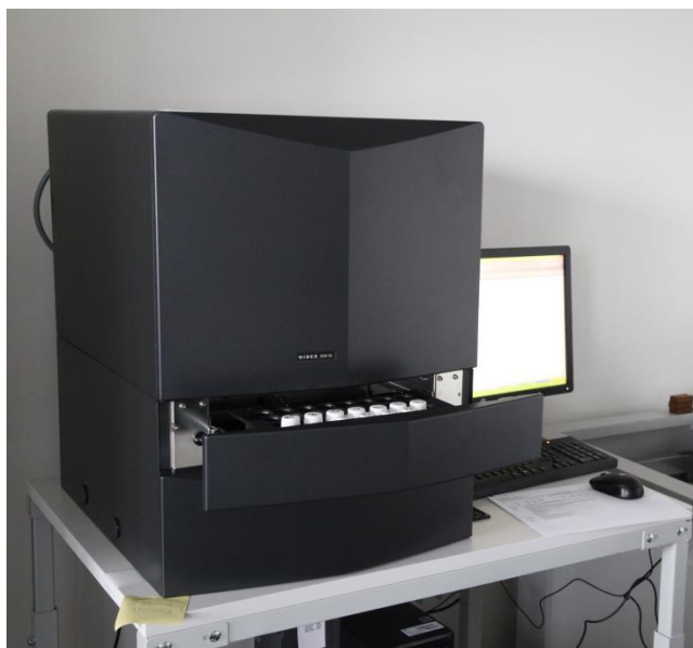
Figure 10: Liquid scintillation counter (LSC) Hidex 300 SL from Hidex OY with TDCR technology.
